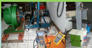
Installation of electrical PMG performance testing
