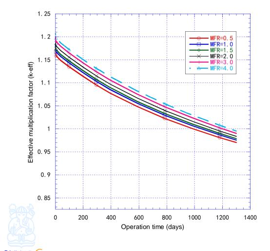
PWR can attain its criticality condition for all MFR values, since k-eff > 1 after more than 2/3 of operation time (cycle length)
