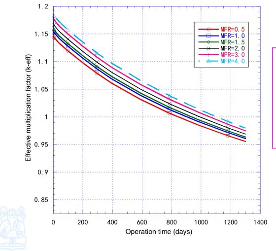
PWR can attain its criticality condition for MFR = 4.0, since k-eff > 1 after more than 2/3 of operation time (cycle length)
