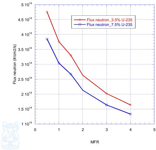
The neutron flux decreases with the increasing of MFR as well as the increasing of UO<sub>2</sub> enrichment in loaded fresh fuel.
