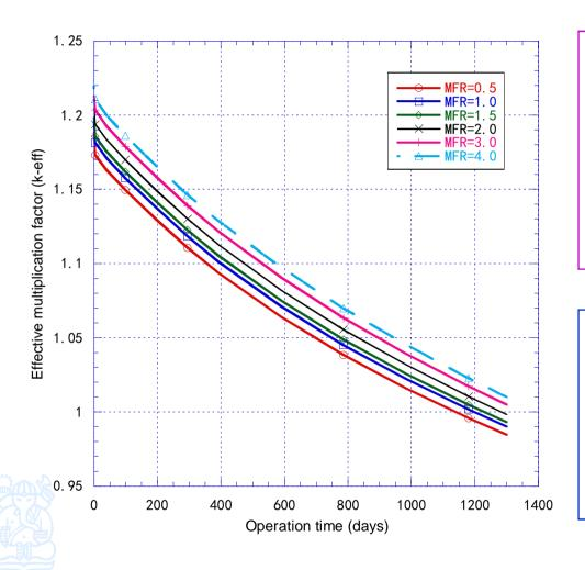
PWR can attain its criticality condition for All MFR values, since k-eff > 1 during the whole operation time (cycle length).
