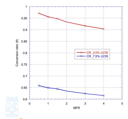
The conversion ratio decreases with the increasing of MFR as well as the increasing of UO<sub>2</sub> enrichment in loaded fresh fuel.
