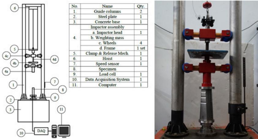
Figure 3 Dropped weight impact testing machine. The instrument used to experimentally test DTDH column as an efficient crush energy absorber.
