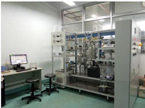
Figure 2 Fixed Bed Micro Activity Test Unit for cracking catalyst activity testing.
