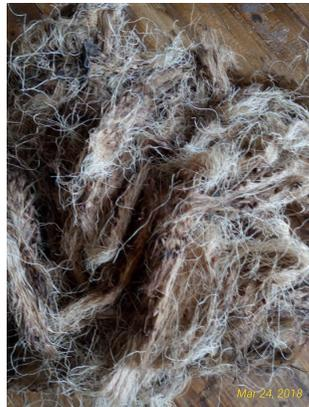
The result of tensile and strength tests shows oil palm EFB fiber has 0.255 kg average strength with 6.160 % ductility in every sheet of the fiber, while the tensile strength and ductility of the oil palm EFB fabric reach 7.928%. Oil palm fiber has high ductility compared to other cellulose fiber such as ramie that has 3-4% ductility.
