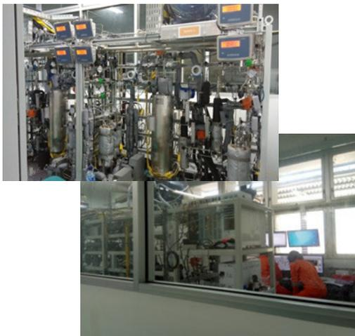
Figure 4 Fixed Bed Micro Activity Test Unit for cracking catalyst activity testing.
