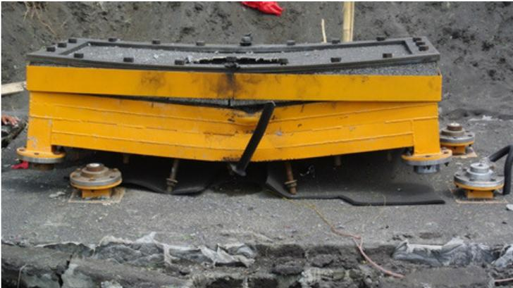
**Figure 1** Experimental testing of Blastworthiness structure; aluminum foam sandwich panel. The explosion test is conducted on February 2018 in PINDAD testing facility
