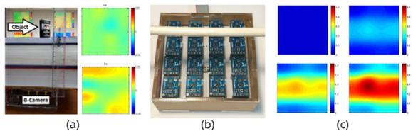
**Figure4** B-Camera, a magnetic field camera: (a) Capability of B-Camera to image an object behind a 12 cm wall, (b) Capability of B-Camera to image a (hidden) powerline cable with various current values. [Source: A.B. Saksmono, D. Danudirdjo, A.D. Setiawan, R.P. Prastio, and D. Rahmawati, IEEE-INTERMAG 2018 Digest]
