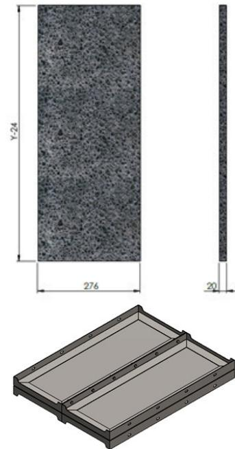
**Figure 6** a) Proposed aluminum foam panel is applied to the train floor structure to reduce the NVH aspects of the railway armada b) attached foam structure to the sub frame
