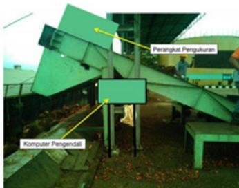
**Figure 1** Illustration of grading sensors in an industrial ramp for individual FFB
