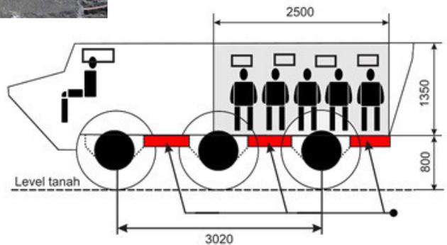
**Figure 2** a) Anoa AFV, modern armoured fighting vehicle is developed by PINDAD b) Modular aluminum sandwich panel location on the Anoa, to deter the landmine explosion
