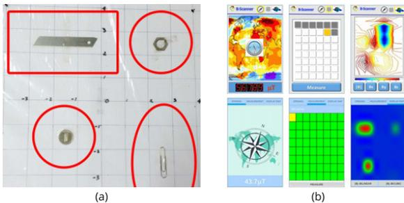
**Figure 3** B-Scanner: Smartphone based (Apps) magnetic field subsurface imaging: (a) Targets placement in test-range, (b) Smartphone screen displaying the Apps and imaging results. [Source: A.B. Saksmono, D. Danudirdjo, A.D. Setiawan and D. Rahmawati, IEEE-Trans. Magnetics, Vol. 53, No. 11, Nov. 2017, 3200405].
