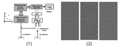
**Figure 2** Compressive SFCW Radar: (1) Block diagram and (2) B-Scan image: original, direct reconstruction, and CS-reconstruction. The number of samples have been reduced 8-times, which means that the data acquisition is 8 times faster. [Source: A.B. Suksmo et al., IEEE-GRS Letters, Vol. 7, No. 4, Oct. 2010]
