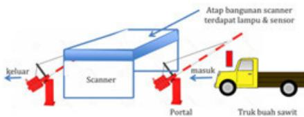
**Figure 2** Illustration of an automatic grading system for a 'per truck' scanning
