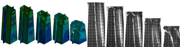
Figure 4 a) Numerical work of DTDH column impact simulation using LSDYNA b) Experimental result of DTDH column, impacted by dropped weight impact testing machine
