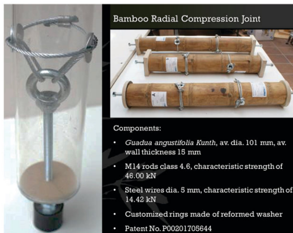
Figure 4. New bamboo joint using new principle: converting tension parallel to the fiber into radial compression force perpendicular to the fiber to the center of its cross section.
