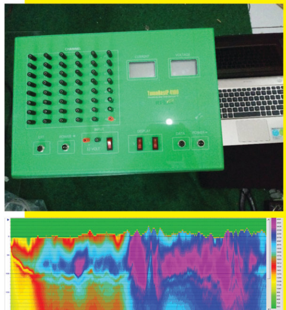
Figure 2. 48 channels Tomography Resistivity - Induced Polarization: Power 1000 watt; Scanned and Controlled by Notebook (PC); Impedance 10 M \Omega ; Bentangan array cable 2D = 1500 meter.
