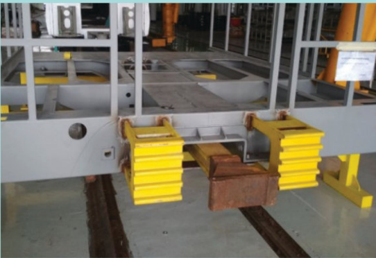
Figure 3. Prototype train underframe equipped with crashworthiness technology.
