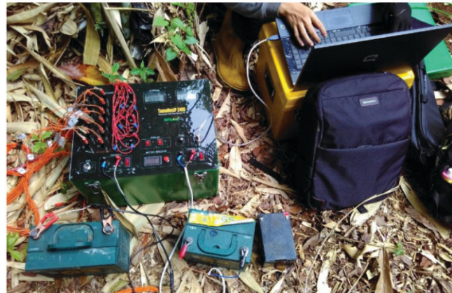
Figure 1. 24 channels Tomography Resistivity: Power 500 watt; Scanned and Controlled by Notebook (PC); Impedance 10 M \Omega ; Bentangan array cable 2D = 300 meter.
