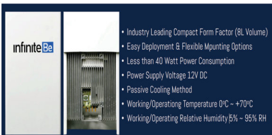
Figure 4. InfiniteBe small cell FSC200 enables mobile service providers to deliver cost-effective capacity to urban hotspots, as well as affordable coverage to rural locations. They also enhance the user experience by enabling faster, more reliable data connections and higher data throughput on 4G networks. FSC200 provides 100 Mbps downlink and 50 Mbps uplink data connections with up to 200 users.
